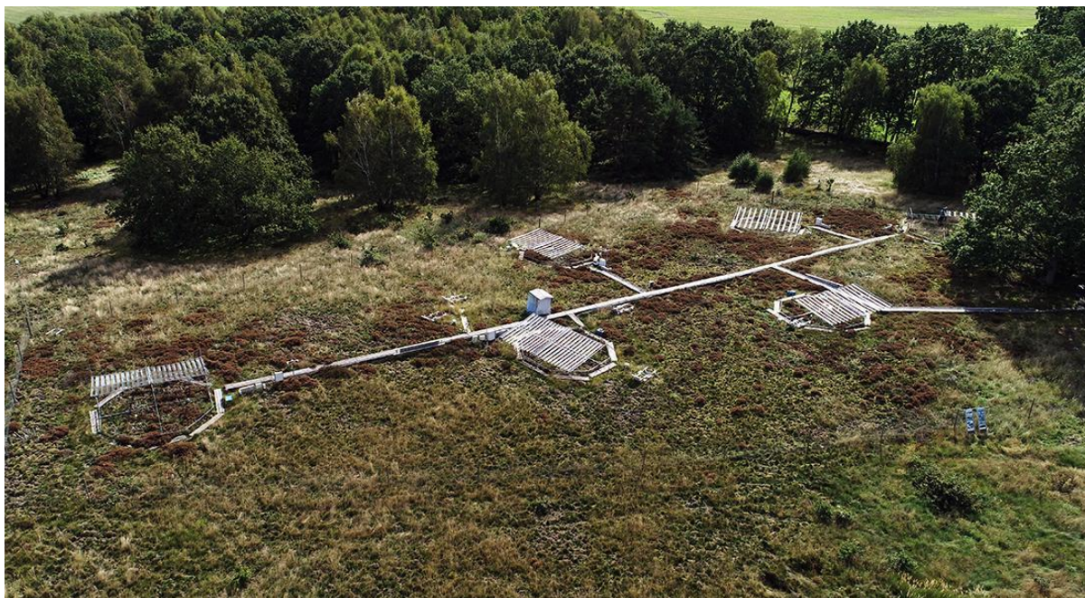
Figure 5. Aerial view of the shrubland/grassland experimental platform Brandbjerg (Denmark). 4 x 8 meter rain-out shelters at 3 different levels of precipitation removal intensity cover the experimental plots (© University of Copenhagen)
