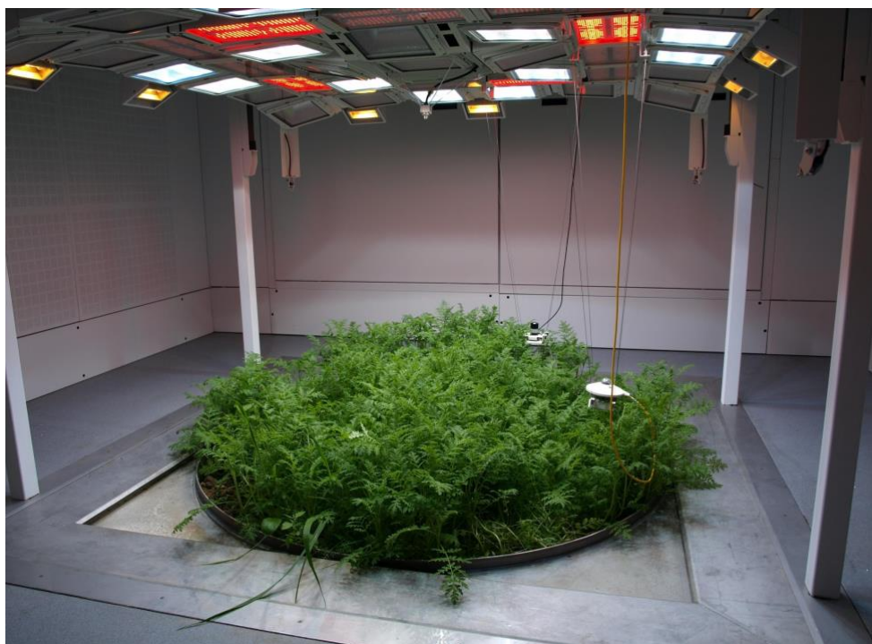
Figure 7. View of a chamber in the Gembloux ecotron (Belgium), featuring the full control of the lightning and heating of the mesocosm (© University of Liège)
