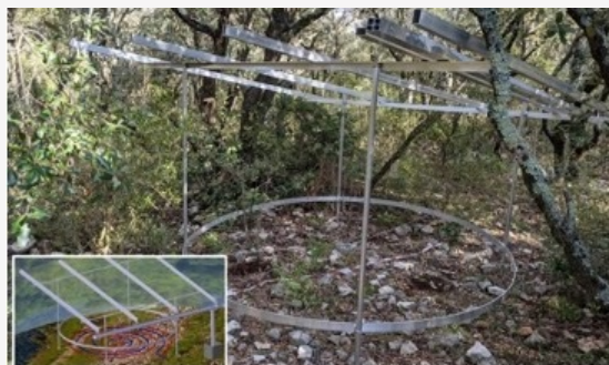
A mobile soil warming and drying experimental device designed at AnaEE France O3HP open-air facility (Ilja Reiter, CNRS).
