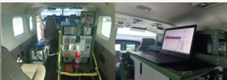
On-board installation of PTR-ToF-MS (model 6000X2; Ionicon Analytik, Austria) for airborne monitoring of volatile organic compounds.
